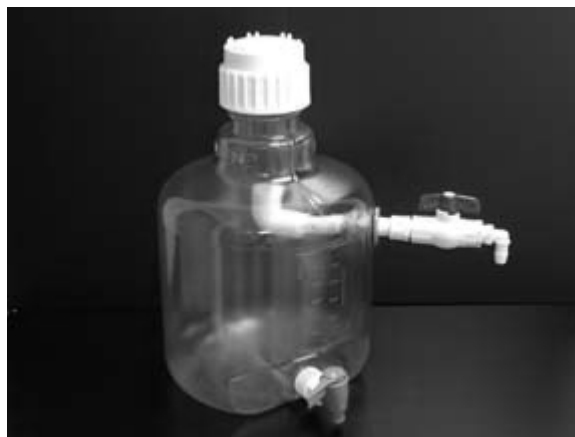
Figure 3. The paramecium collector is made from a carboy, with a spigot at the bottom, and various plumbing fixtures (Fig. 4). A 16 liter carboy is recommended for larger facilities, although an 8 liter carboy will work well for those needing to make only small amounts of paramecia.
