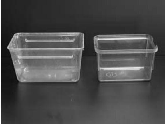
Figure 1. The container on the left is a polycarbonate Nalgene animal cage (24x14x13 cm). It has a volume of approximately 2 liters. The container on the right is a Thoren crossing cage and holds approximately 1 liter. Both containers work well for paramecia and any similar containers should be adequate.
