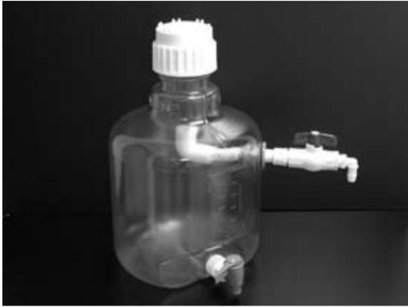
*Figure 3.* The paramecium collector is made from a carboy, with a spigot at the bottom, and various plumbing fixtures (Fig. 4). A 16 liter carboy is recommended for larger facilities, although an 8 liter carboy will work well for those needing to make only small amounts of paramecia.
